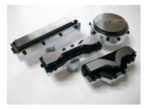
The Dumbbell cutting knife is a cutting knife with easily replaceable cutting blades. This new generation of cutting knife is ideal for producing highly accurate test bars, resulting in better and more consistent results. Each cutting knife includes a built-in extractor as well as 5 sets of replacement cutting knives, replacement screws and the associated tooling.
