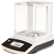
An analytical balance with a digital display and a glass enclosure. | Analytical balance | H3000     |
