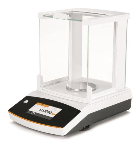
The analytical balance is required in every test laboratory. It is used to precisely determine important values such as MFR, carbon black content, K-value, degree of crosslinking, OIT, volatile matter, water absorption, etc.
